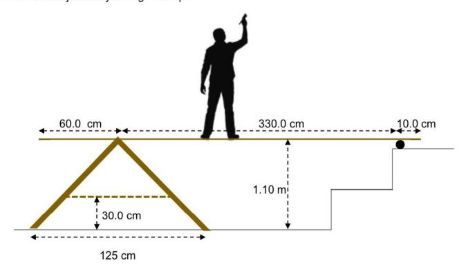
(a) If the center of mass of the painter is directly above the center of the trestle, calculate the force exerted by the edge of the step on the plank.
